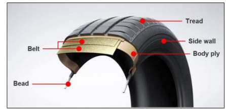
The structure of tires Source: Bridgestone website
